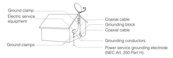
Note: If the Satellite/Antenna cable is grounded correctly (as specified above), connecting it to the DIRECTV $^{\textcircled{R}}$  DVR will properly ground the DVR. The DVR must be properly grounded before you connect it to a telephone line, and it must remain grounded thereafter.
